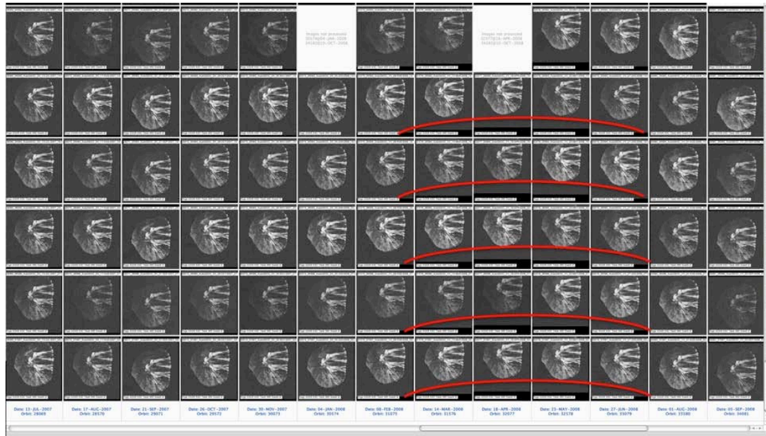
Figure 6: Extract of web tool showing coherence maps of the Fogo volcano, Cape Verde. (Fogo Ascending Track 460 Swath i2). The scenes are always processed with the same crop counted in lines and pixels in the Master image. One can clearly see the shift of the volcanic island in the frame of the scene as underlined by the red curves.
